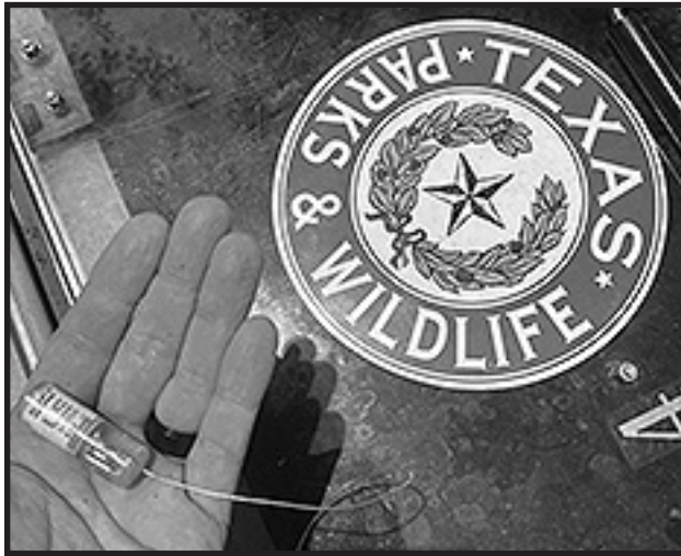
Telemetry device inserted into bass to study tracking and behavior.
